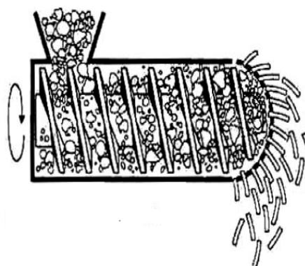
Fig. 1: Axial Screw feed extruder
