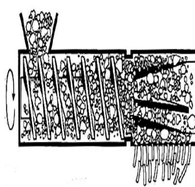
Fig. 2: Radial Screw feed extruder
