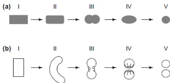
Fig. 8: Pellet-forming mechanism according to: (a) Rowe – I) Cylinder; II) Cylinder with rounded edges; III) Dumb-bell; IV) Ellipse; V) Sphere. (b) Baert – I) Cylinder; II) Rope; III) Dumb-bell; IV) Sphere with a cavity outside; V) Sphere.<sup>28</sup>
