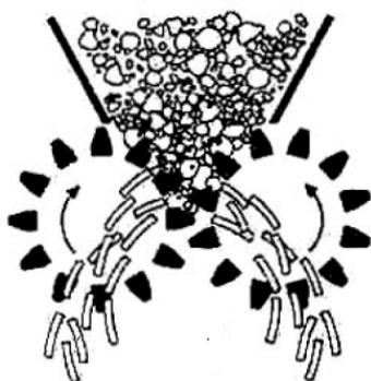
Fig. 6: Gear roll type
