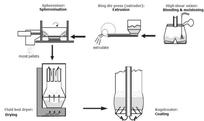
Fig. 9: Extrusion-spheronization process.
