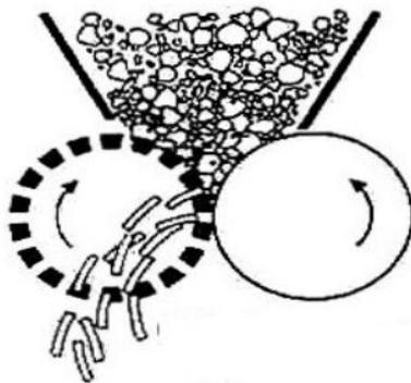
Fig. 5: Cylinder roll type
